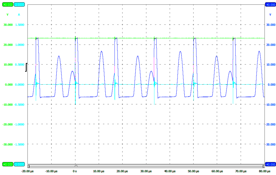
Figure 28: Instability of coil 5 at 60 kHz, alternating state.
